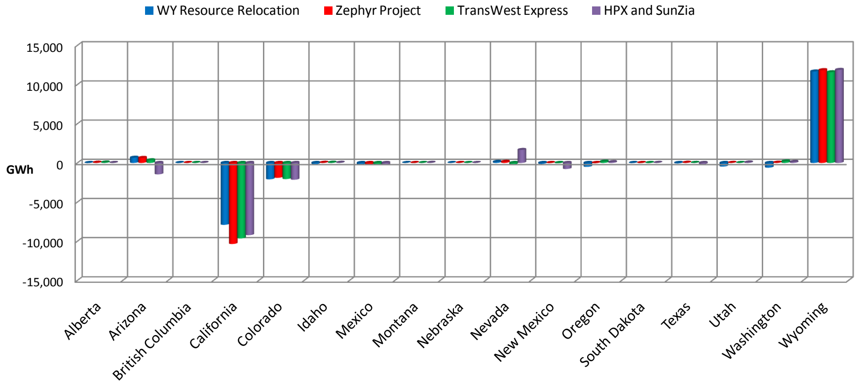
Change in Annual Generation by State - WY Resource Relocation and Transmission Expansion Cases Compared to PC1A Base Case
